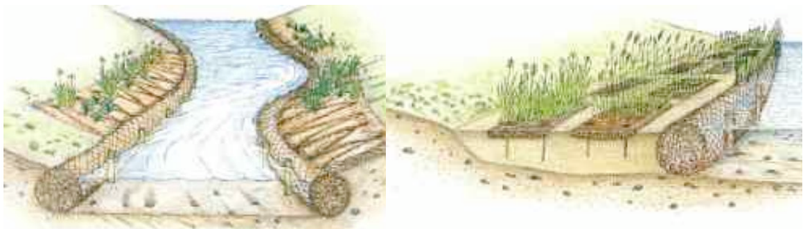
Fig. 1: Schematic application of BGS Pregrown Fibre Rolls™ and mats for erosion protection along river banks
